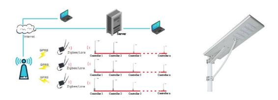
All In One Solar Street Light system integrated with **Solar panel,LED lamp, intelligent controller** and A grade **Li-FePO4 battery** packing. It's together with/without motion sensor, offers a solution of low-energy consumption, long-lasting and high-Luminance as well as free maintenance for at least 6-8 years. The all in one solar street light working mode can be adjusted according to different control requirement. Also it could provide convenient transportation and installation.
